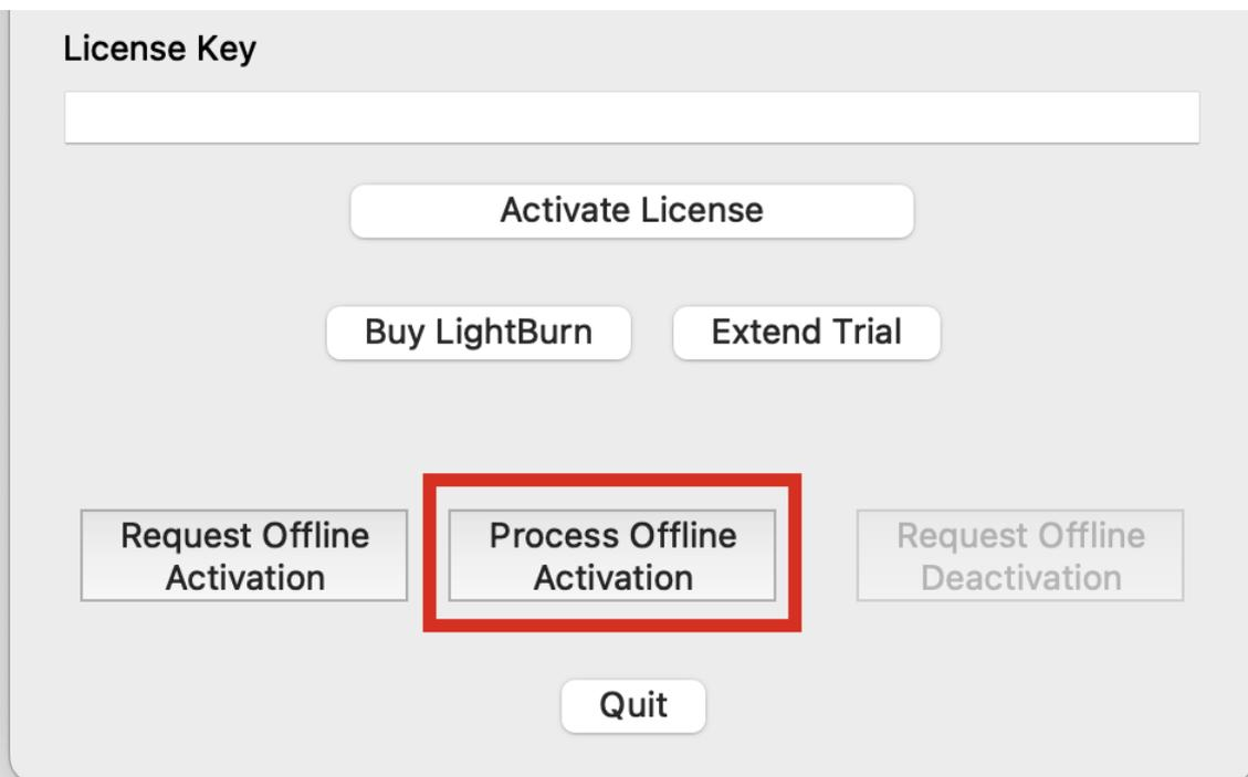
8. Navigate to the location the .dat response file is saved and select it, completing the Offline Activation process.
