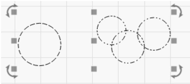
Ungrouped objects are displayed with a simple dash pattern when selected, like the single circle above on the left. A grouped shape shows a repeating dot-dot-dash pattern when selected, shown on the three smaller circles above on the right.
