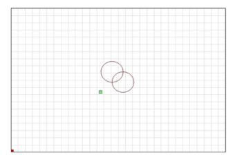
Notice that the green Job Origin indicator has moved. This represents the position of the laser when you start the job, so the laser is going to move slightly up and to the right from wherever it is, cut the two circles, and go back to where it started.
