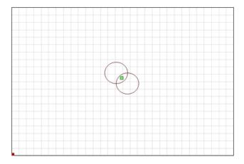
The job will be centered around the current position of the laser head. If you position the laser head directly over the center of the item you want to etch, the output will be centered on the item.
